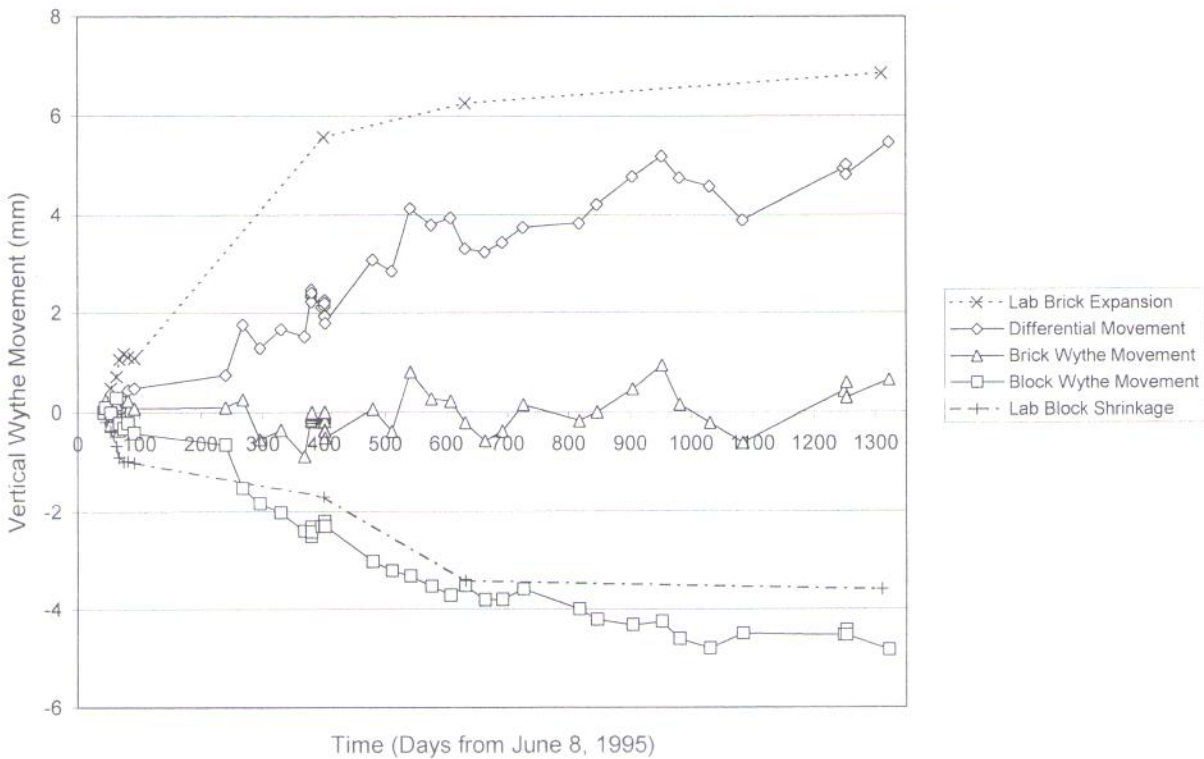
Figure 9 - West Cavity Wall Wythe Movement with Thermal Movements Removed (Cavity wall details: Shear transfer ties, 100 mm wythe spacing, 50 mm rigid insulation)
