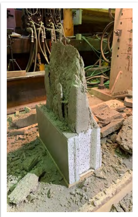
Prism specimens post test.
