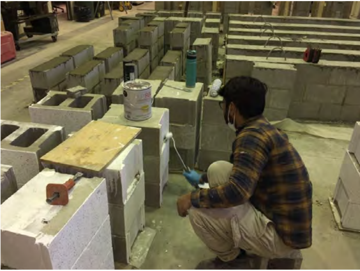
Nitesh applying a white paint and speckle pattern so that the Digital Image Correlation equipment can track the deformation of the prisms under load.
