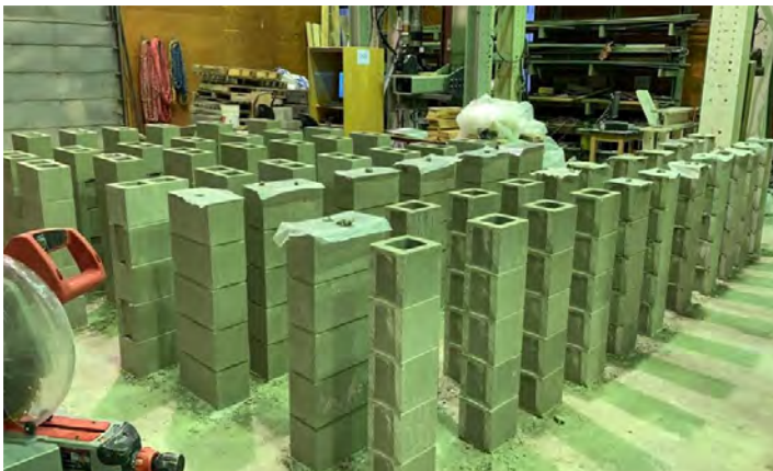
Gordon is comparing testing standards for masonry prisms between the Canadian CSA S304 and American ASTM C1314 by testing various prism configurations.
