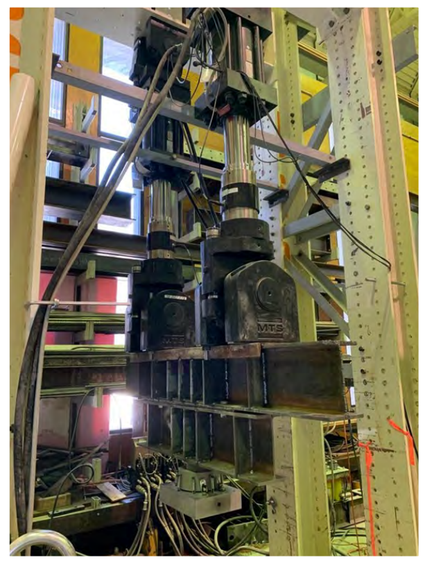
Two actuators, capable of exerting 1000kN each (about 225 000lb-f) had to be coupled together in order to have the necessary capacity to test the prisms.
