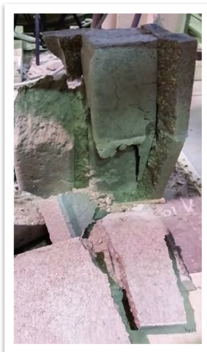
Prism specimens post test.
